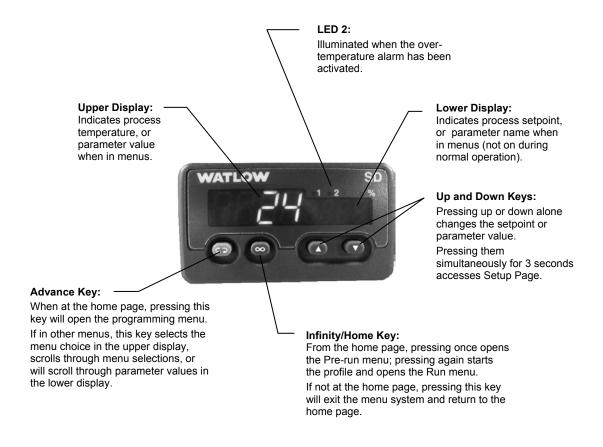
Figure 2 Limit module keys and displays
